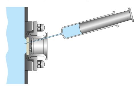
Note that the correct Steriflange must be used with the Long sample port in order to ensure proper sealing of the membrane.
